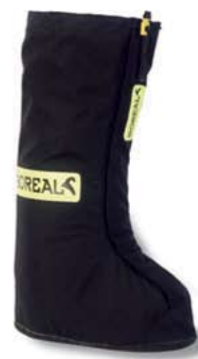
► 440 Expe over boot Triple layer Thinsulate® lined over gaiter with EVA sole. Outer of Cordura backed with Sympatex® for high abrasion resistance, waterproofing and breathability. All seams are thermosealed for absolute protection. Cold spots are eliminated by placing the Thinsulate® in the gaiter without the use of glue or stitching. The gaiter is manufactured according to GI Expe boot size and Left / Right, to ensure a perfect fit and maximum thermal efficiency. This makes The Expe Over Boot / GI Expe combination the finest system available for 8000m ascents in winter and conditions of exceptional cold.
